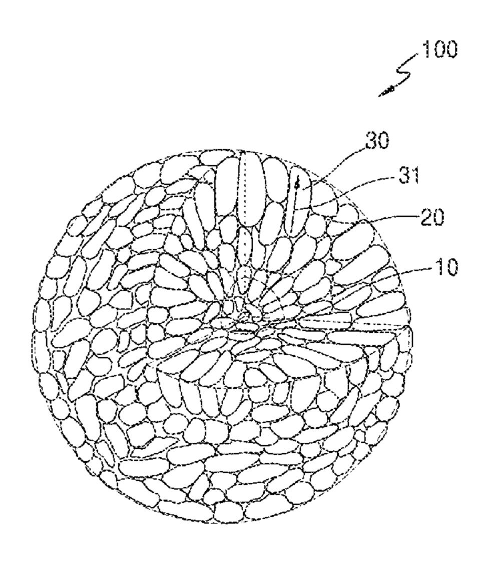
distance, in which intercalation and deintercalation of lithium are facilitated, may be obtained. A lithium secondary battery manufactured using the positive active material may exhibit enhanced lithium availability, and may exhibit enhanced capacity and lifespan due to suppression of crack formation in the active material during charging and discharging.
