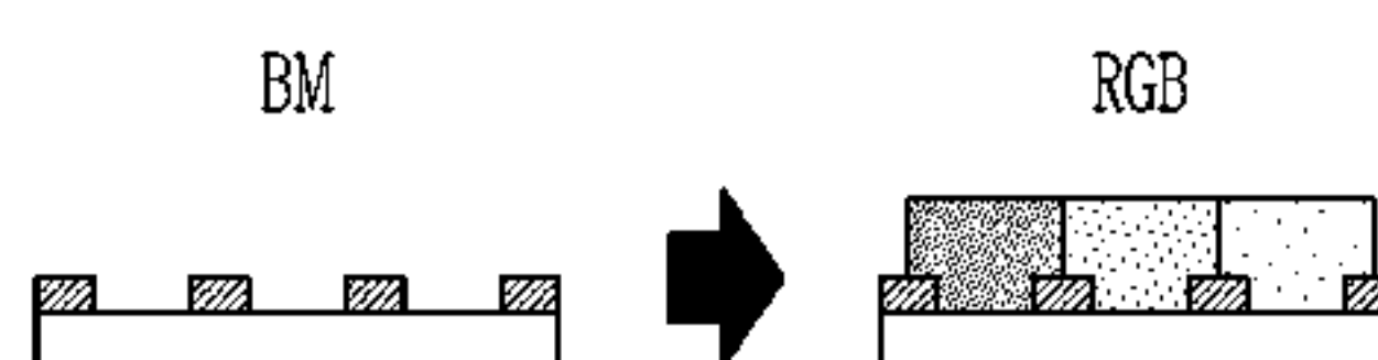
Repeating the Patterning Process three times
