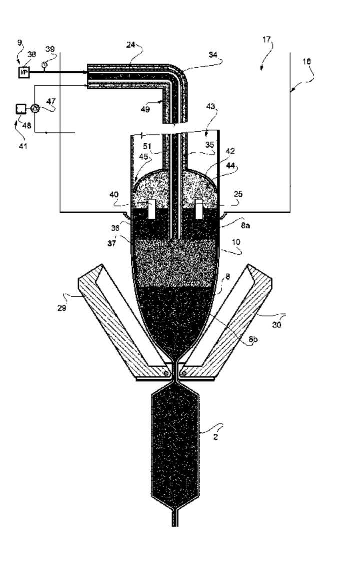
filling, a sterile gas into the product column for forming and/or maintaining a gas cushion within the product column.
