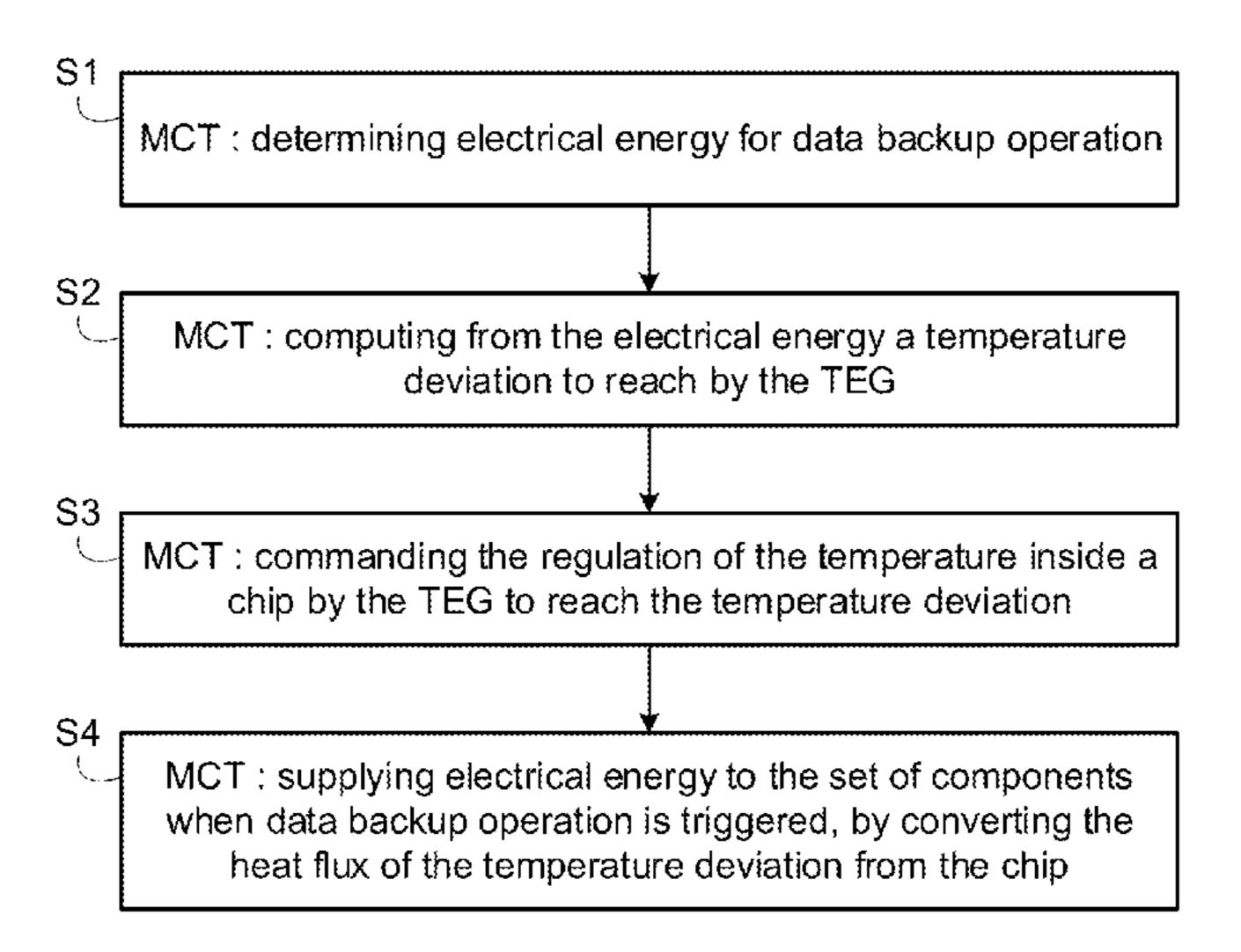
wherein the microcontroller is configured to command the regulation of the temperature inside the chip by means of the thermoelectric generator to reach the temperature deviation, wherein the microcontroller is configured to supply electrical energy to the set of components when data backup operation is triggered, the electrical energy being converted from the heat flux of the temperature deviation from the chip.
