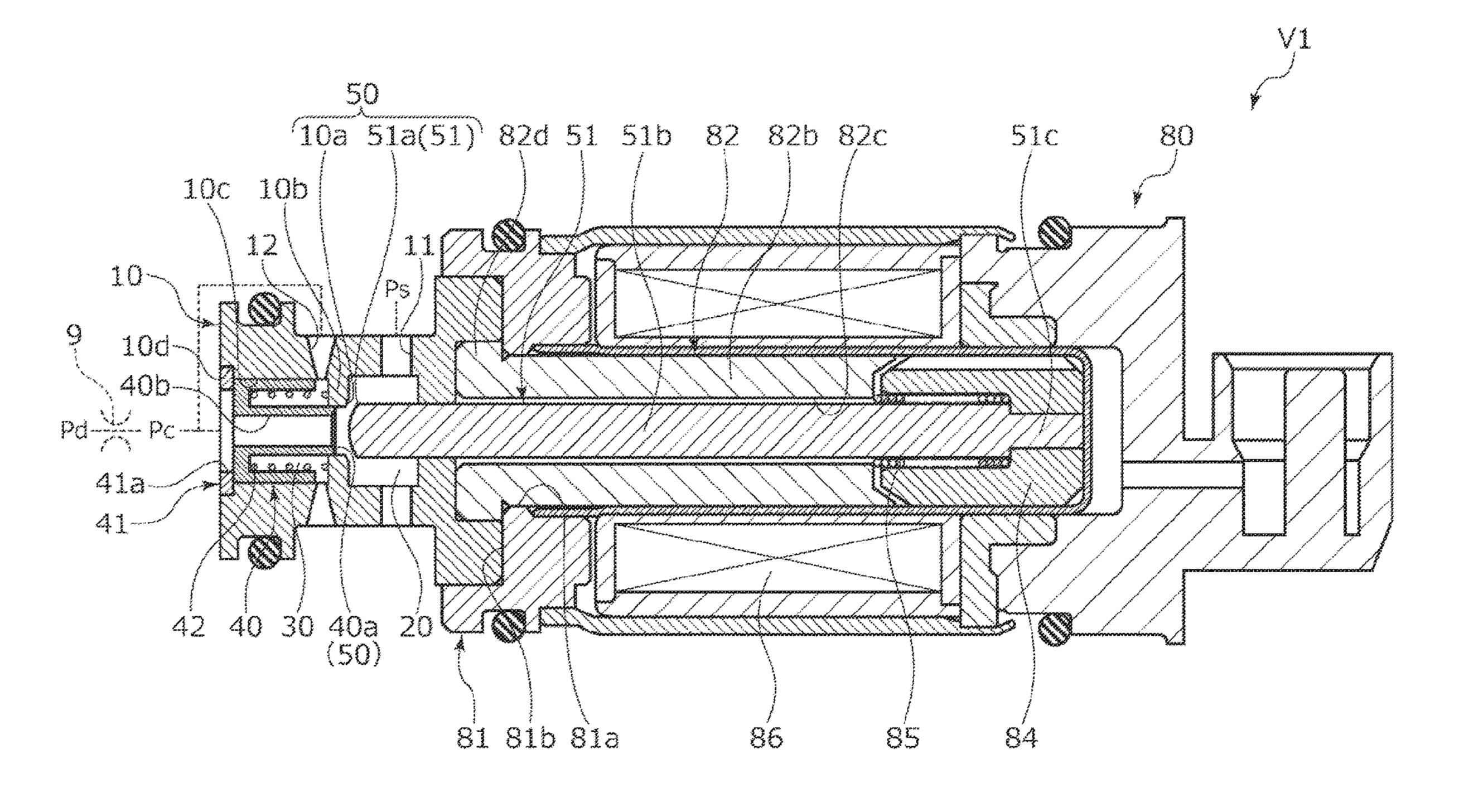
configured for moving in a direction toward the valve body due to a differential pressure between a primary pressure and a secondary pressure.
