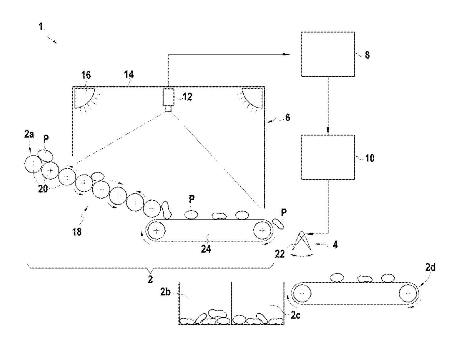
products on themselves, mounted in the conveying unit facing the image acquisition unit, and configured to allow an exposure to the image acquisition unit, of the different parts of the conveyed agricultural products.
