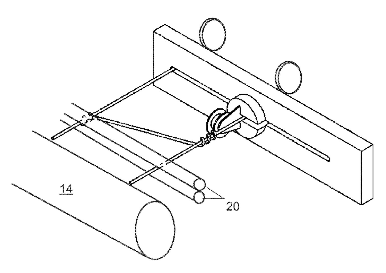
mined path of the crossing wire from the additional wire spool forms the weave with the longitudinal wires from the wire spools.
