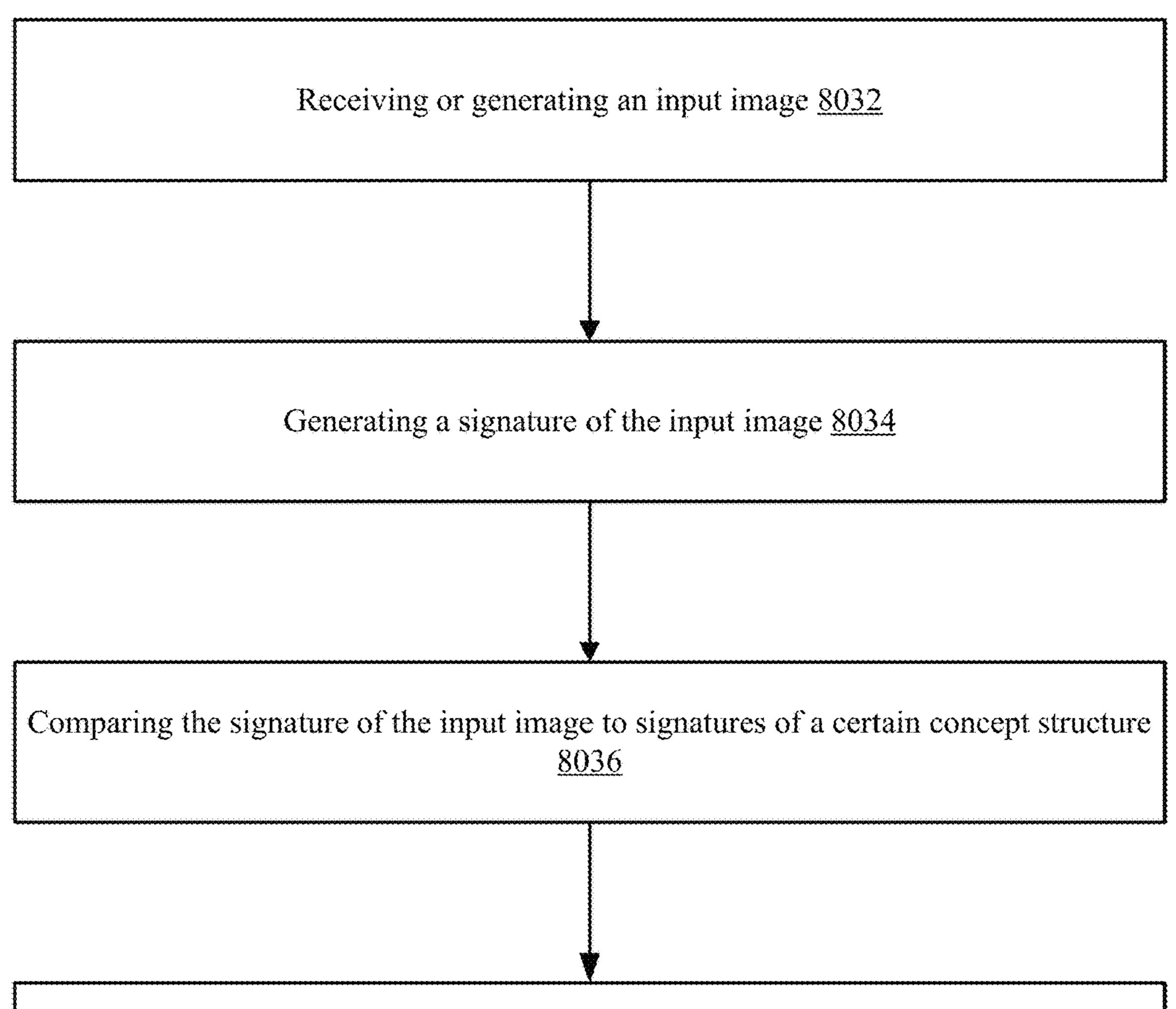
Determining that the input image comprises the object when at least one of the signatures of the certain concept structure matches the signature of the input image <u>8038</u>
