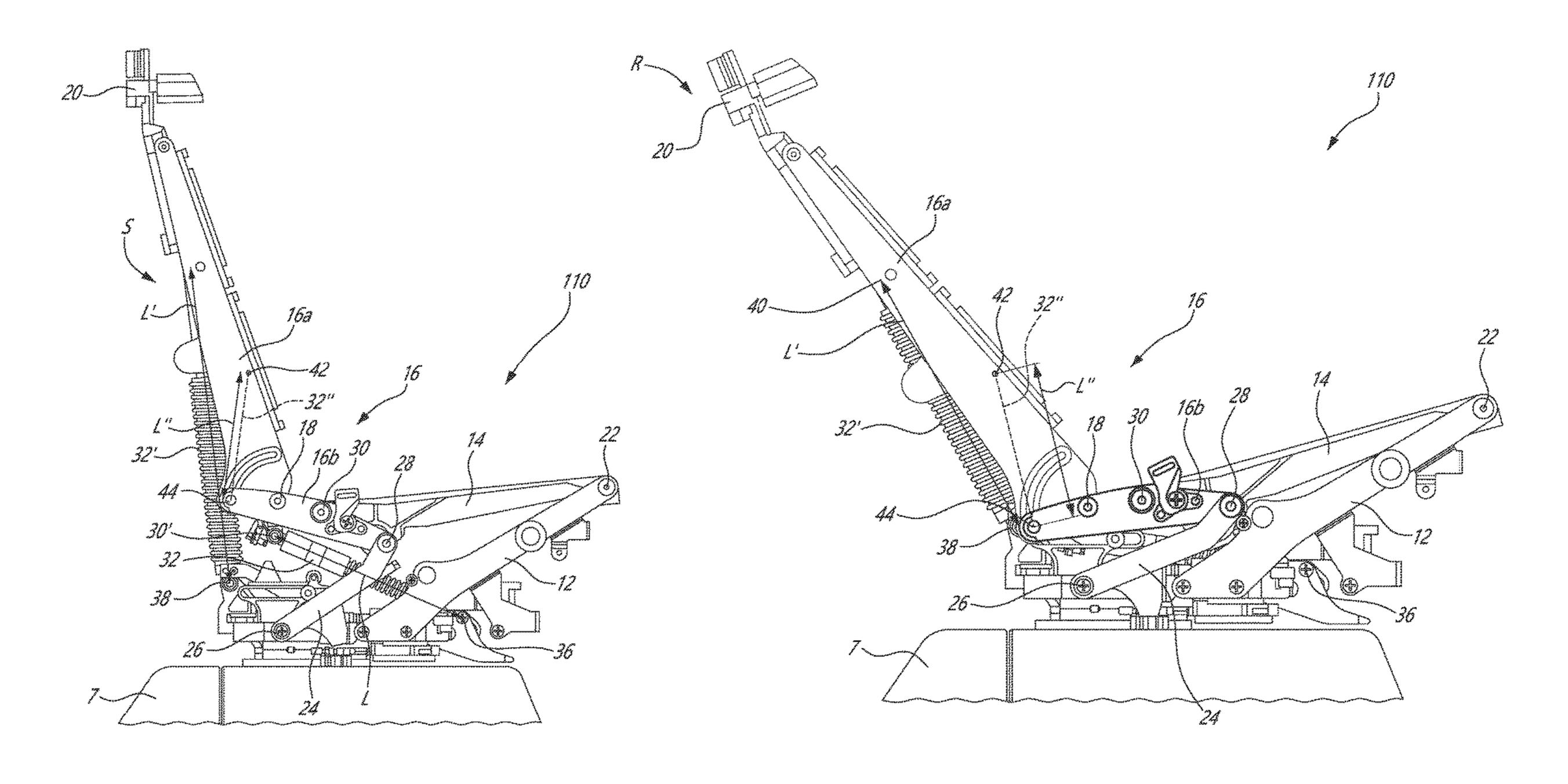
pivots and about the first and second locations. The length of the backrest linear actuator is substantially the same in the reclined configuration and in the berth configuration.
