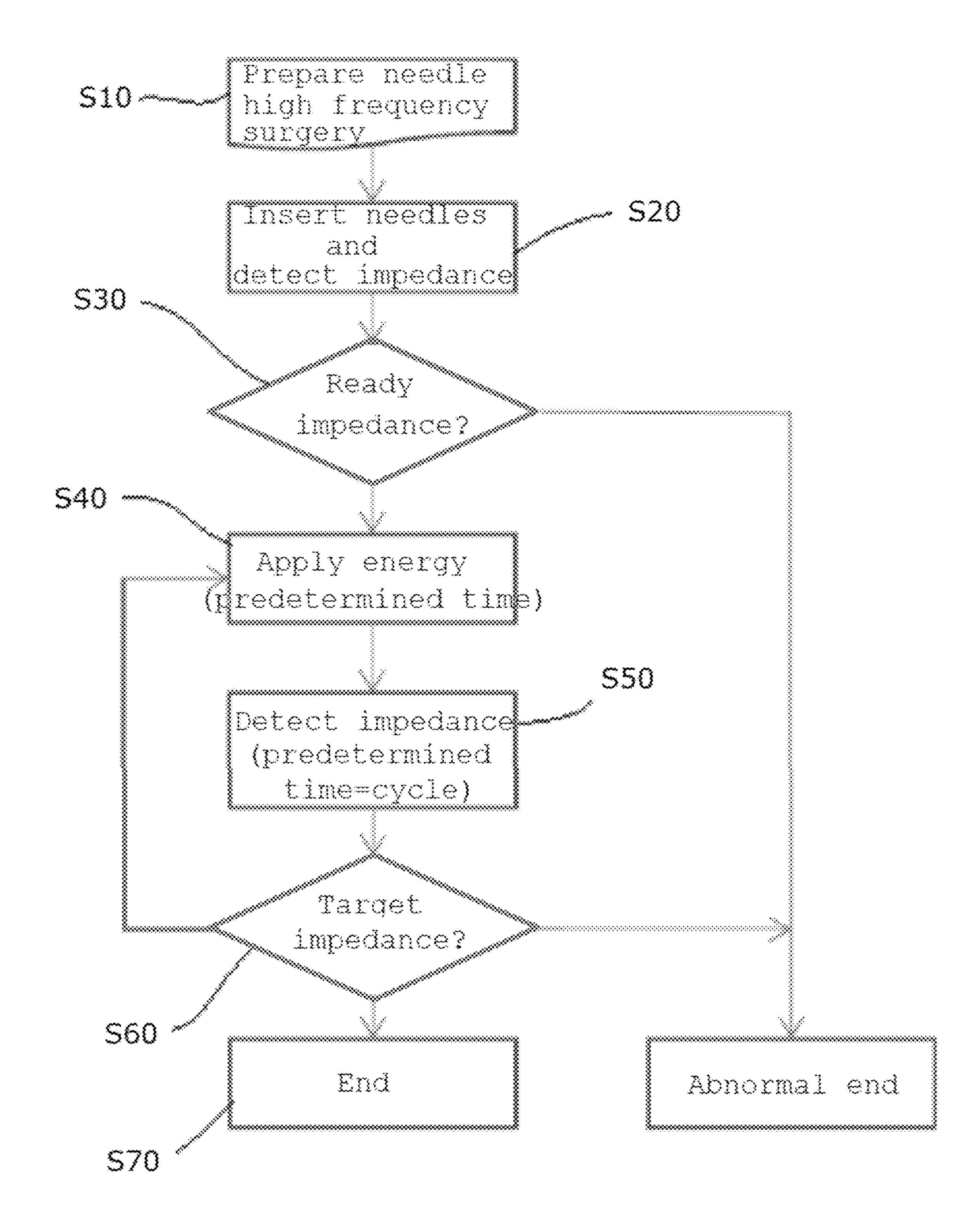
SURGICAL NAVIGATION INSTRUMENT HAVING NEEDLE ELECTRODE DEPTH ADJUSTING STRUCTURE FOR DETECTING IMPEDANCE AND HIGH FREQUENCY ENERGY CONTROL METHOD USING SAME
