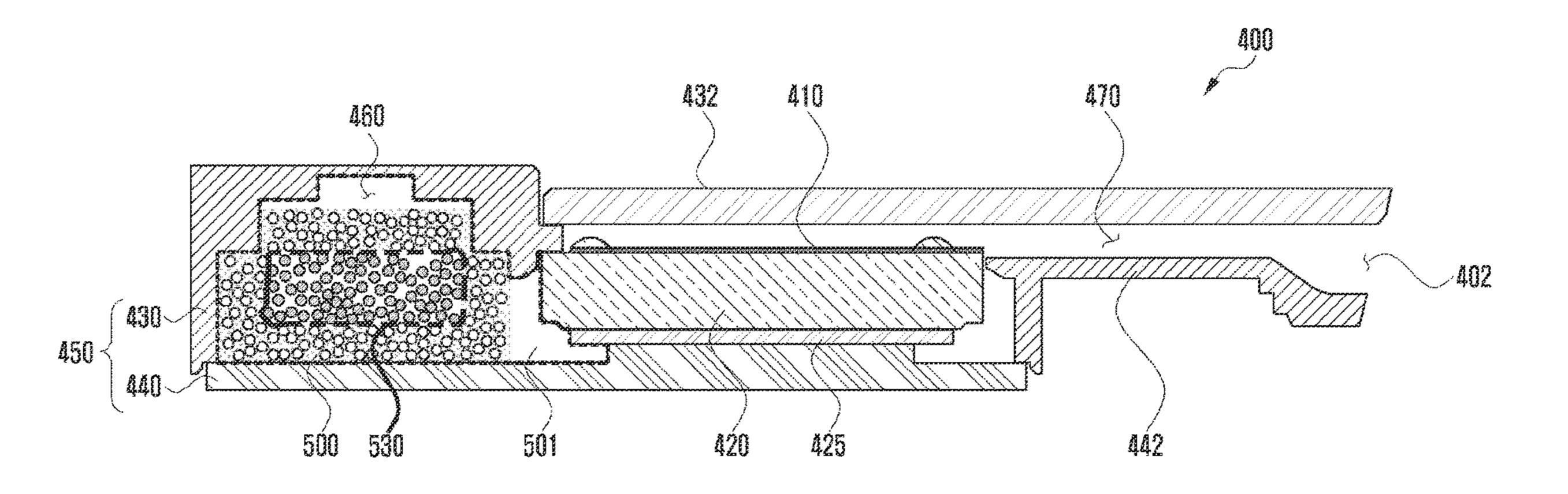
direction from the speaker module and a second space provided in a second direction opposite the first direction. The electronic device further includes an air adsorption member comprising an air adsorbing material disposed in the first space and having a volume ratio of 90% or less of the first space, the air adsorption member configured to reduce air resistance to the diaphragm disposed above the speaker module without limiting the vibration of the diaphragm.
