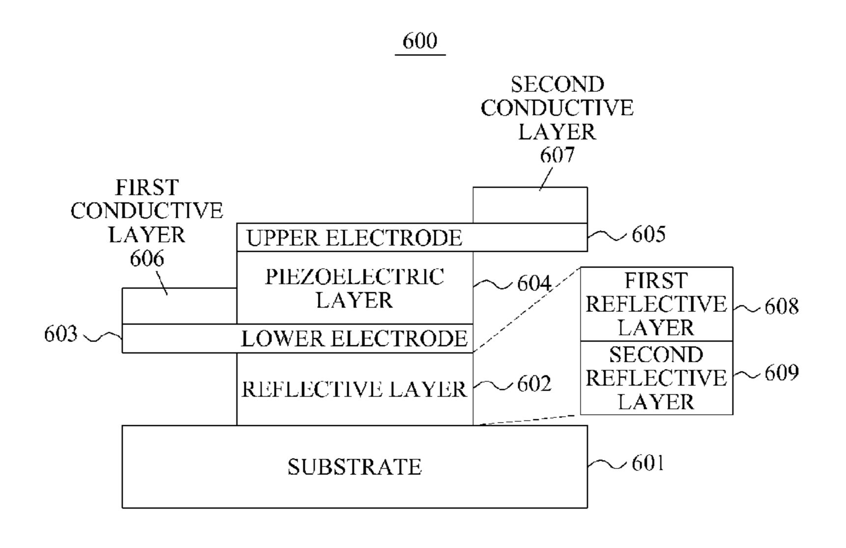
includes an upper electrode formed on the piezoelectric layer, and a conductive layer formed on the upper electrode or the lower electrode.
