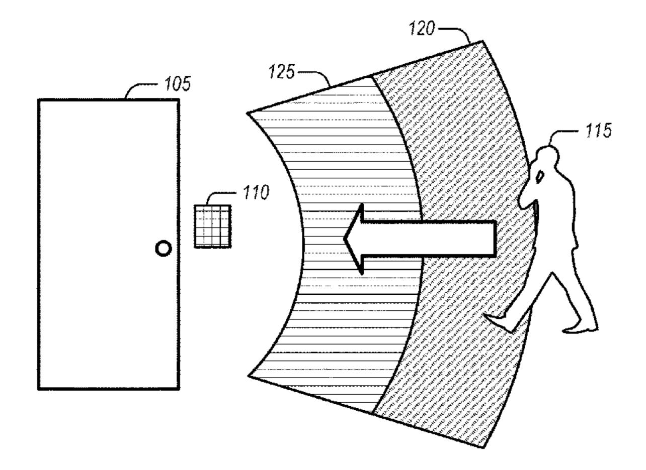
connection with the key device. The access control system may be further adapted to request a validation of the credential from an authorization service in response to establishing the second wireless connection with the key device. The access control system may receive a validation token from the authorization service. The access control system may be further adapted to store the validation token in the cache.
