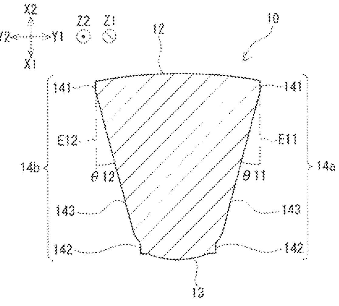
a protruding portion projecting outwardly from the peripheral surface of the first member, and the first member, the second member, and the third member are configured by an integrally molded green compact.
