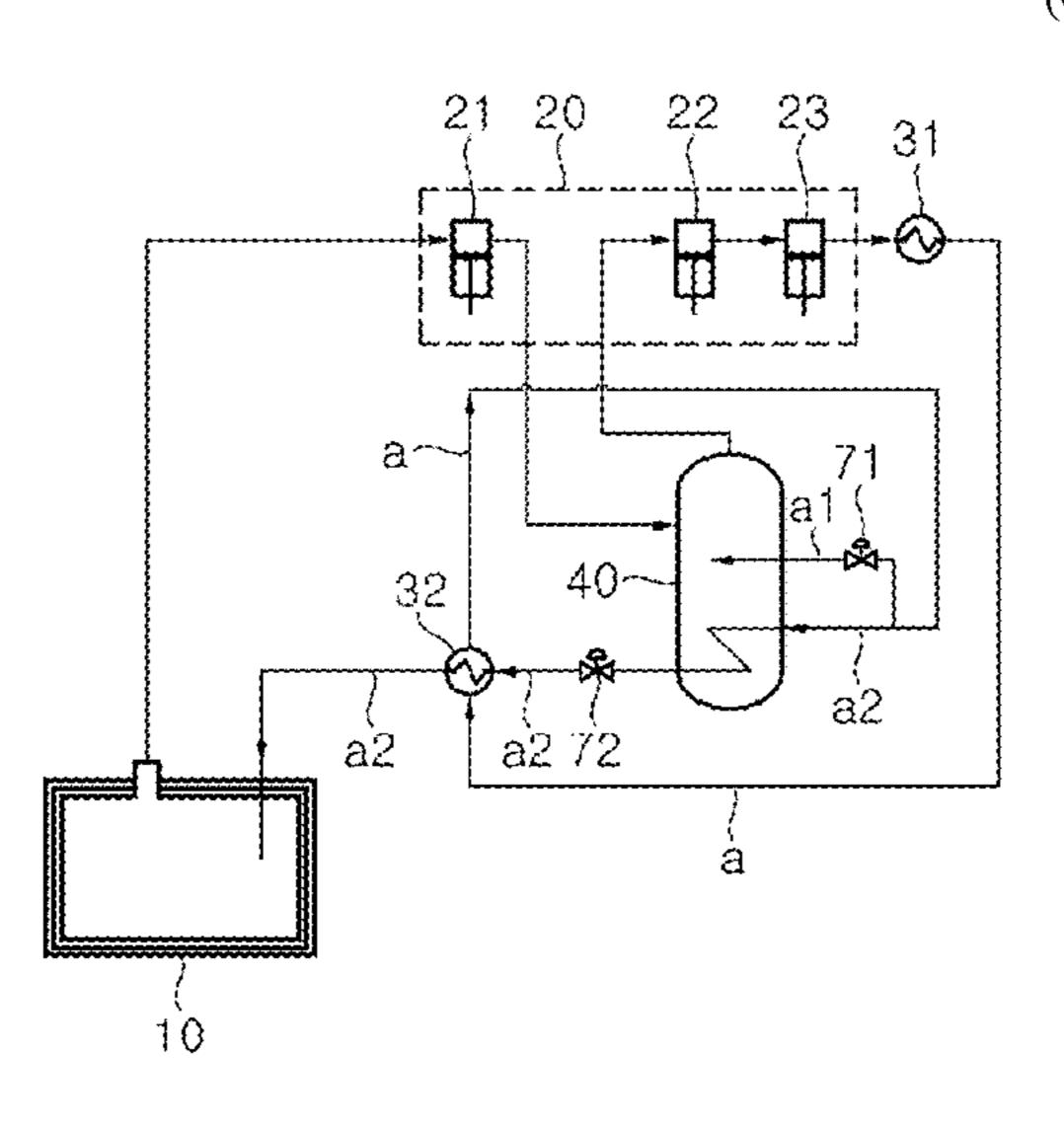
and thus cooling same; and a second decompressing device for expanding "flow a2" which has been cooled by the third heat exchanger.
