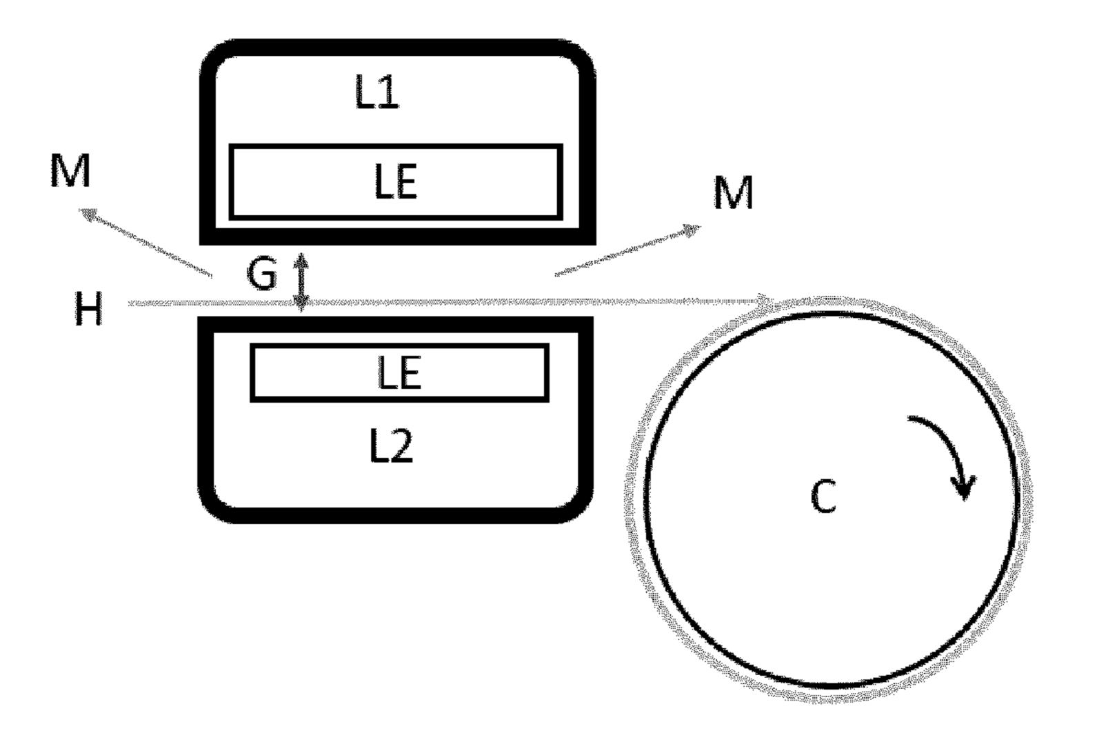
measurement. The sensors may be arranged for measuring an areal light density profile of a whole treatment area. The hair styling device may radiate hair from two sides, both of which includes an areal light absorption measurement. The sensors may include LEDs that do not produce light.
