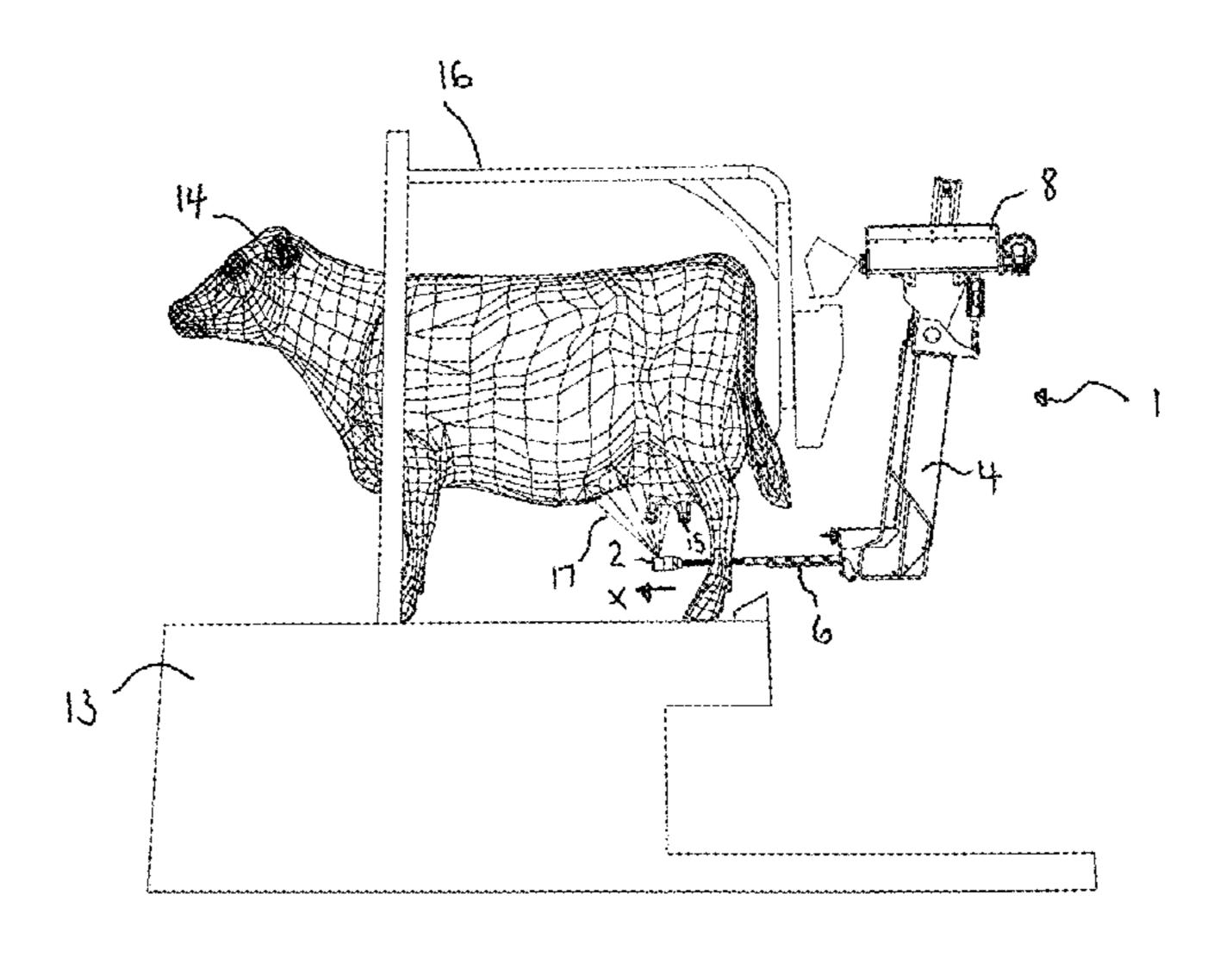
configured to actuate spraying of the animal's teats from spray nozzle extension and retraction in response to a signal received from the sensor.
