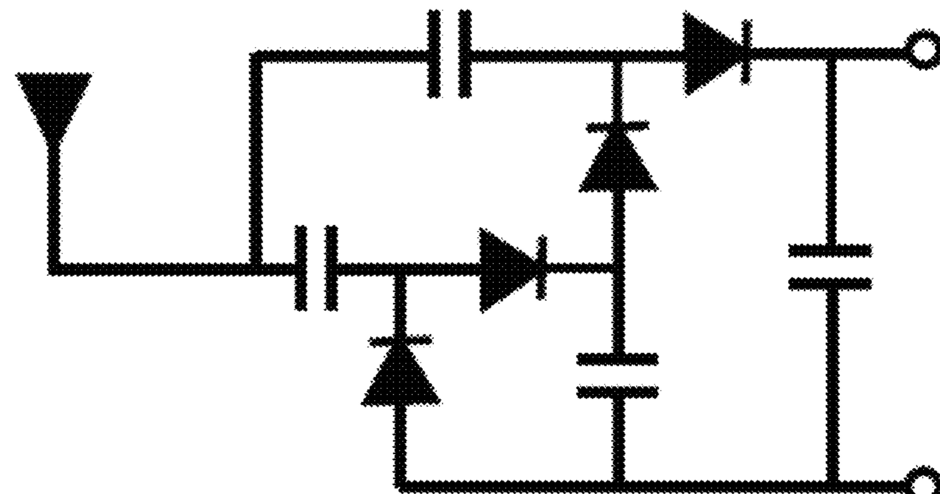
**Charge-pump & Capacitor****FIG. 7A****FIG. 7B**
