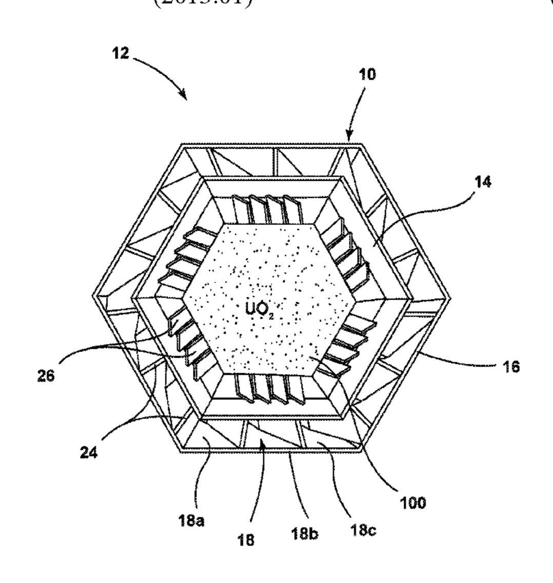
swelling of the nuclear fuel, for example UO<sub>2</sub>, when undergoing fission. The nuclear fuel cladding is formed according to an additive manufacturing process, for example laser powder bed fusion printing.
