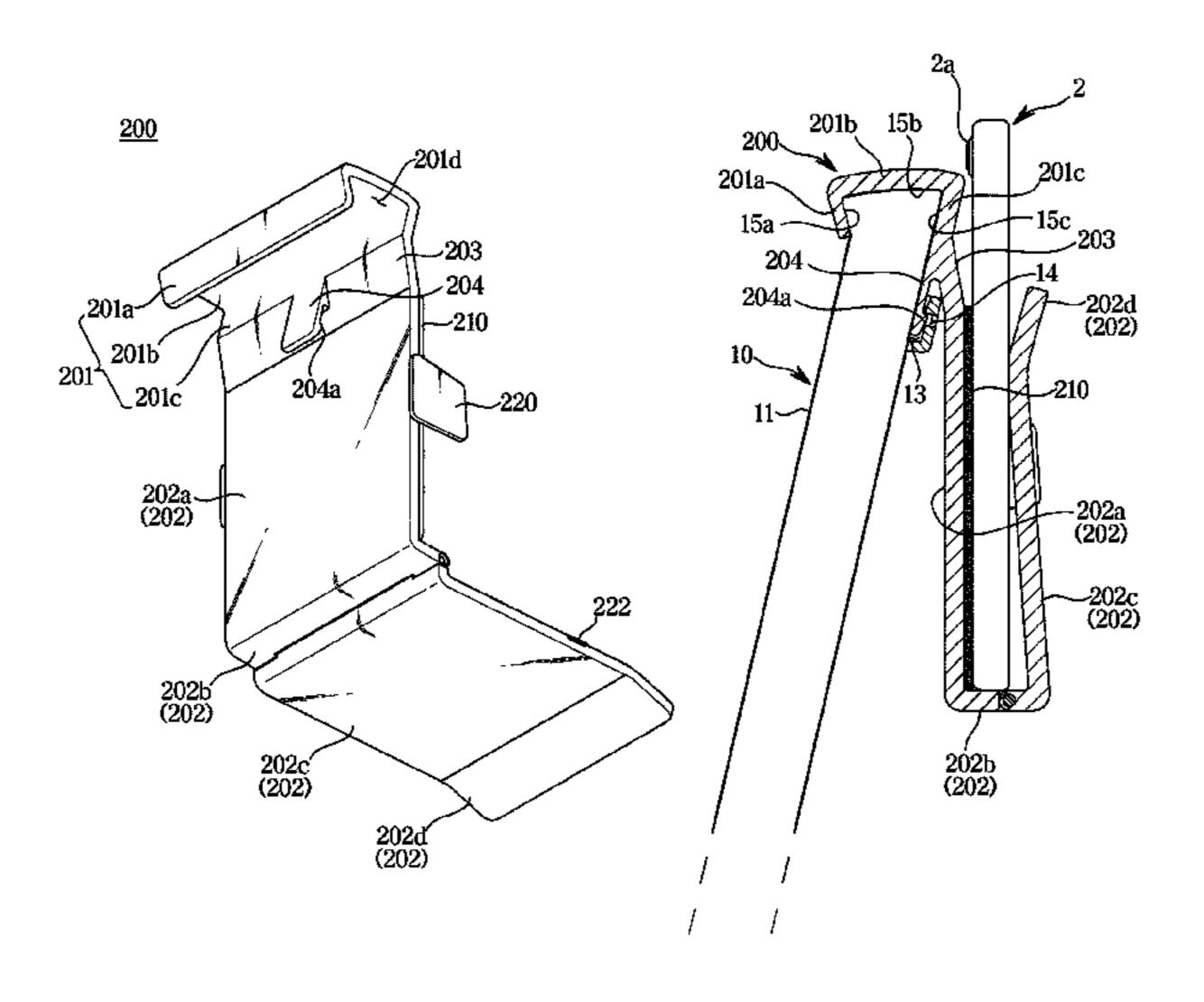
mounting portion, and accommodates the mobile device such that the mobile device is mounted on the display module.
