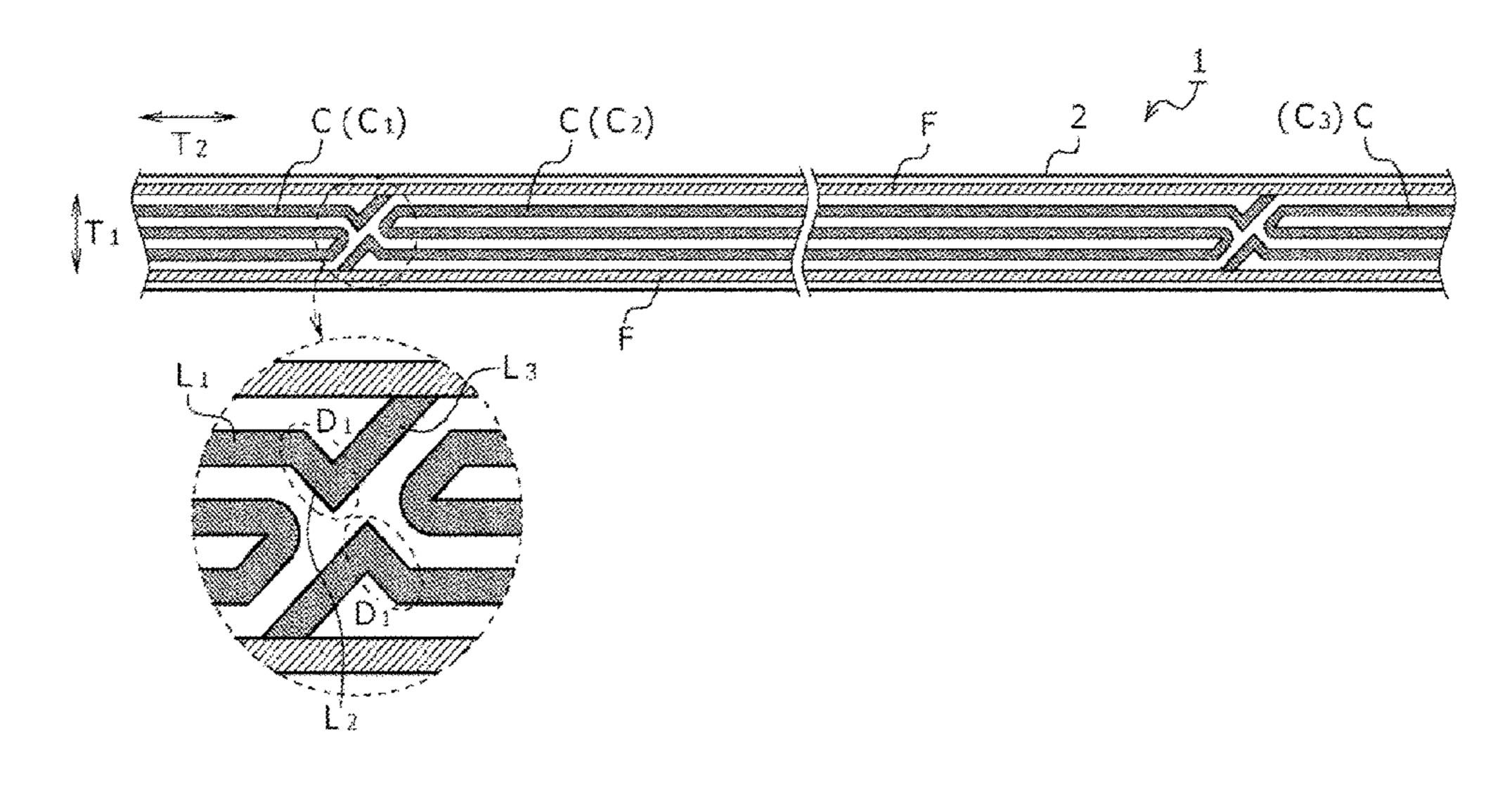
extending in substantially parallel with the longitudinal direction of the base and a plurality of oblique wires tilted relative to the lateral wires.
