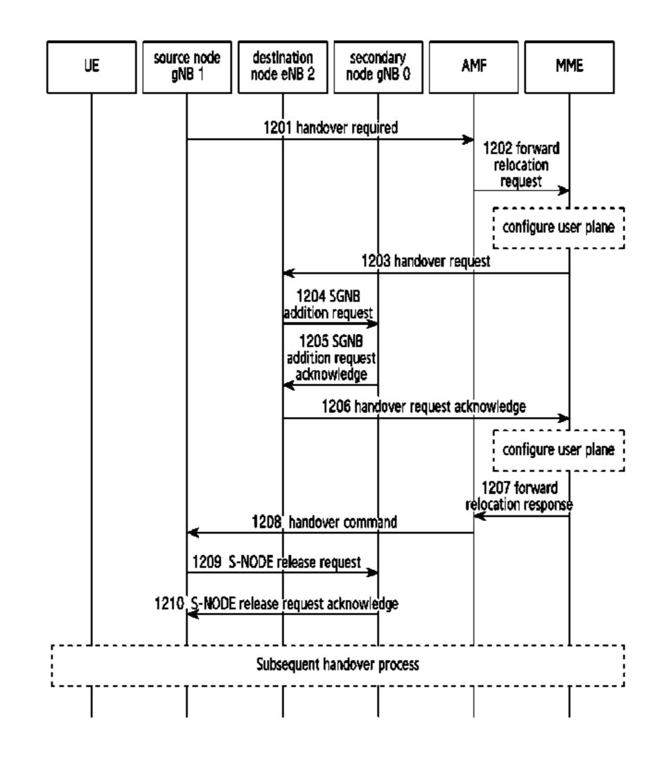
request message for the inter-system handover from the EPS to 5GS with the SgNB used as the target gNB; and receive, from the target gNB, an acknowledge of the handover request message. The handover required message includes an SgNB user equipment (UE) X2 application protocol ID (SgNB UE X2AP ID) for identifying a UE over X2 interface in the SgNB. The handover request message includes the SgNB UE X2AP ID, and the SgNB UE X2AP ID is allocated at the SgNB.
