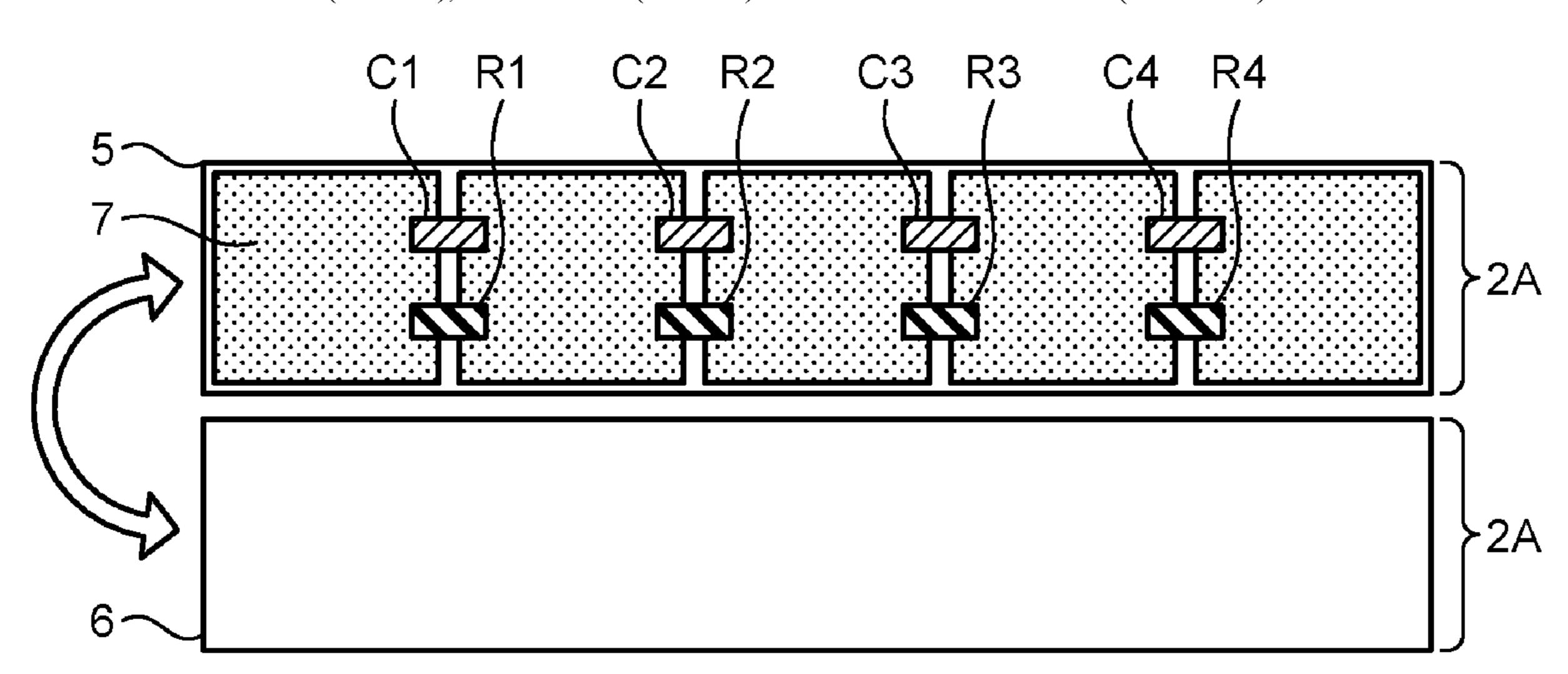
resistive voltage dividing board face each other and that the conductor patterns arranged on the front face of the one resistive voltage dividing board are disposed oppositely from the conductor patterns arranged on the front face of the other resistive voltage dividing board.
