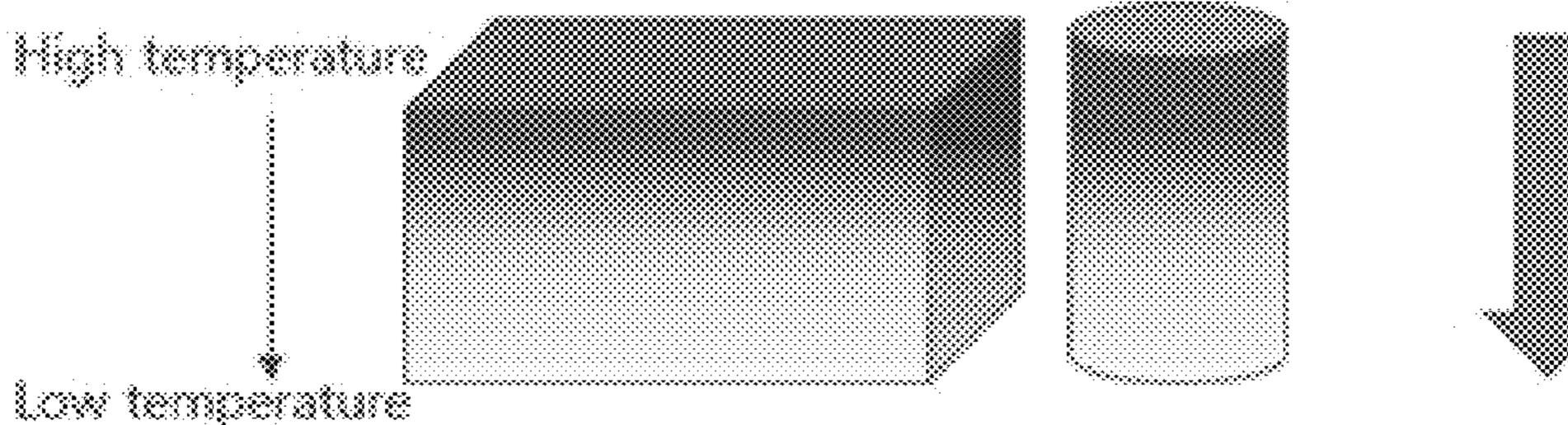
Appling graded heattreatment temperature to make functionally graded materials Direction of high transmittance and low flexural strength
