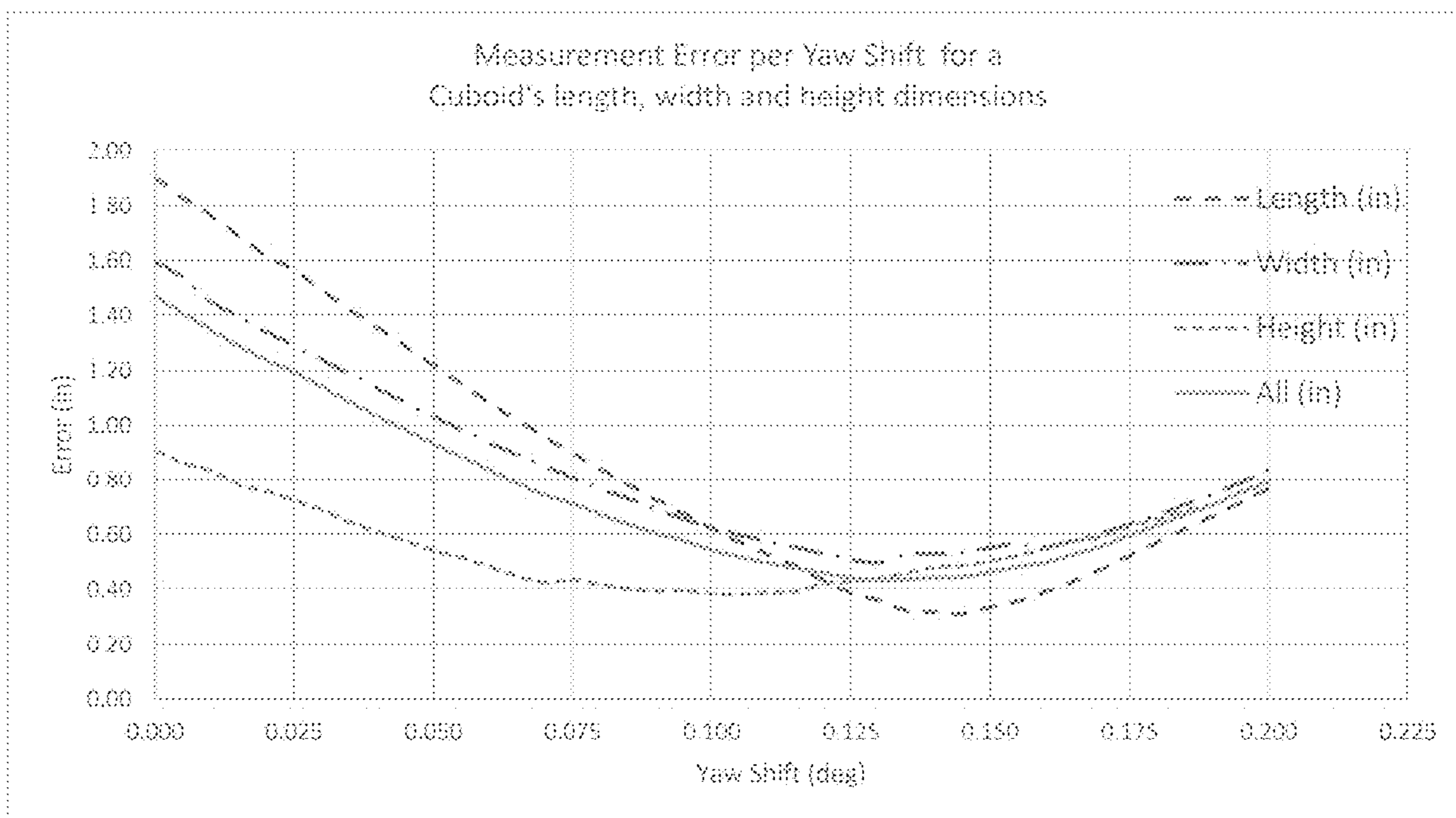
Figure 12: Dimensioning error minimization by modification of yaw parameter
