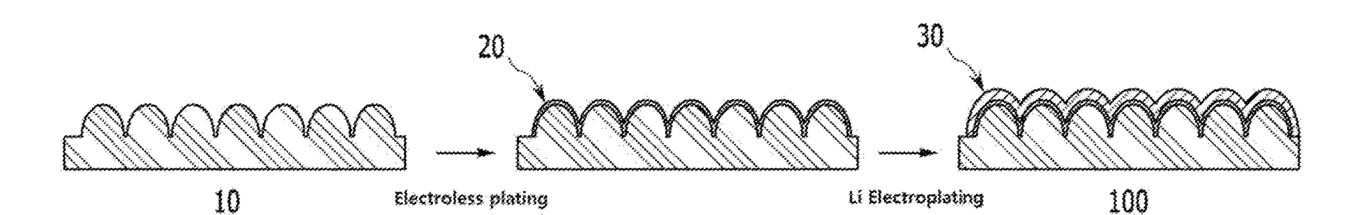
and an active material layer, thereby improving processability during manufacture of the electrode and assembling the battery.
