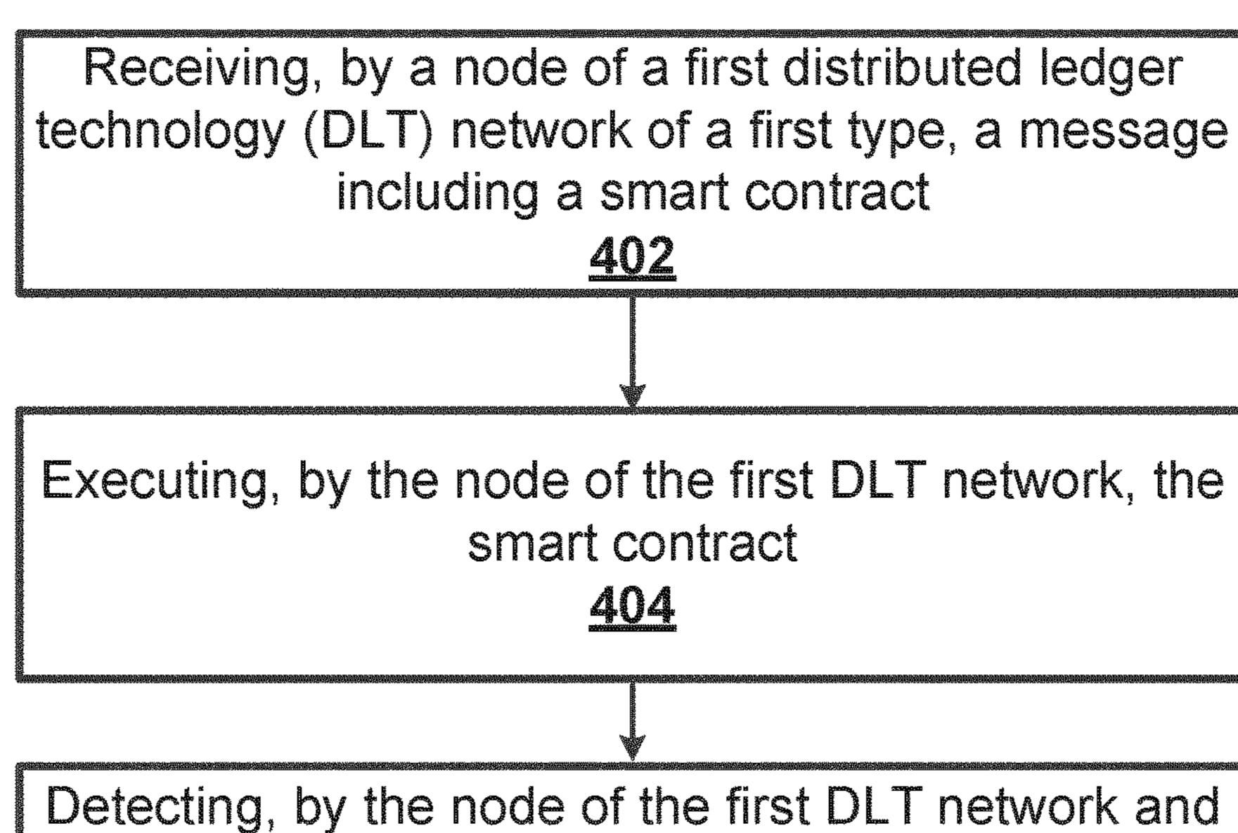
via the smart contract, a transaction request to transfer a digital currency from the first DLT network to a second DLT network of a second type
