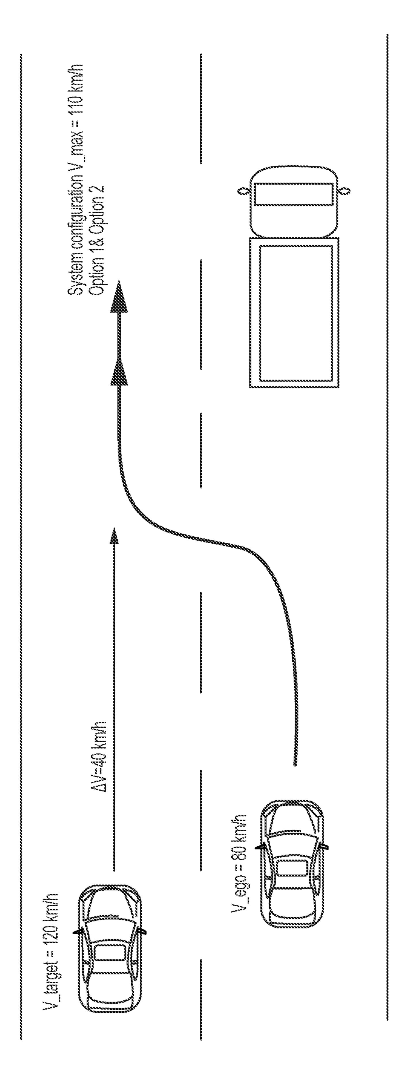
Option 1: Accelerate to adapt with V\_target and execute lane change fully automatically Option 1a: Driver is able to trigger the lane change maneuver Option 1a: Driver is able to trigger the lane change maneuver Option 2: Display V\_target proposal to driver -> manual acceleration and manual lane change.
