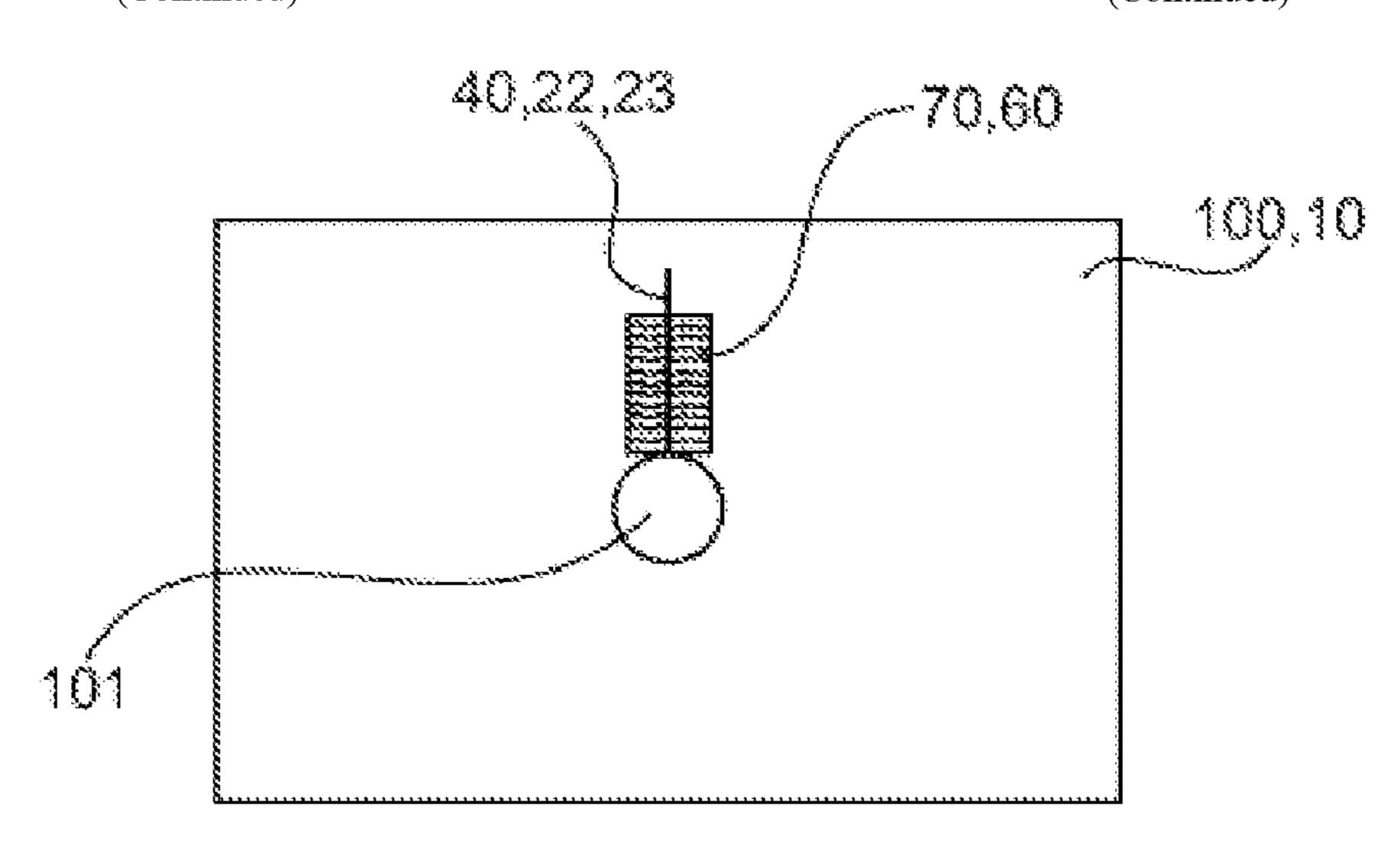
extruded part and is connected to the extruded part such that the fiber grid bridges the two material inner edges. The extruded part may be a part of a battery housing for a traction battery.
