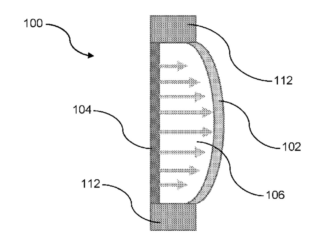
layer (102) is stretched by the actuation element while the inelastic fabric layer (104) is undeformed.
