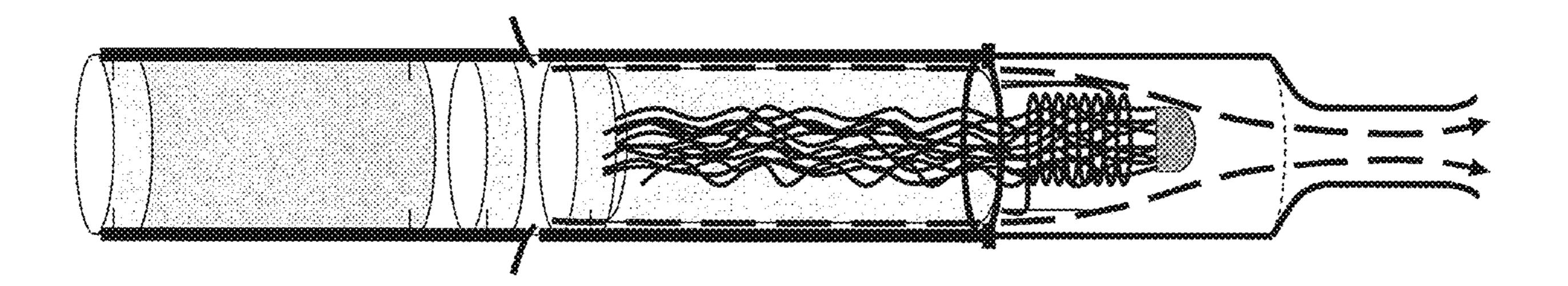
use, liquid is transferred from the liquid storage portion towards the heating element by capillary action in the wick. Liquid at the second end of the capillary wick is vaporized by the heating element. The supersaturated vapor created, is mixed and carried in the air flow from the at least one air inlet to the aerosol forming chamber. In the aerosol forming chamber, the vapor condenses to form an aerosol, which is carried towards the air outlet.
