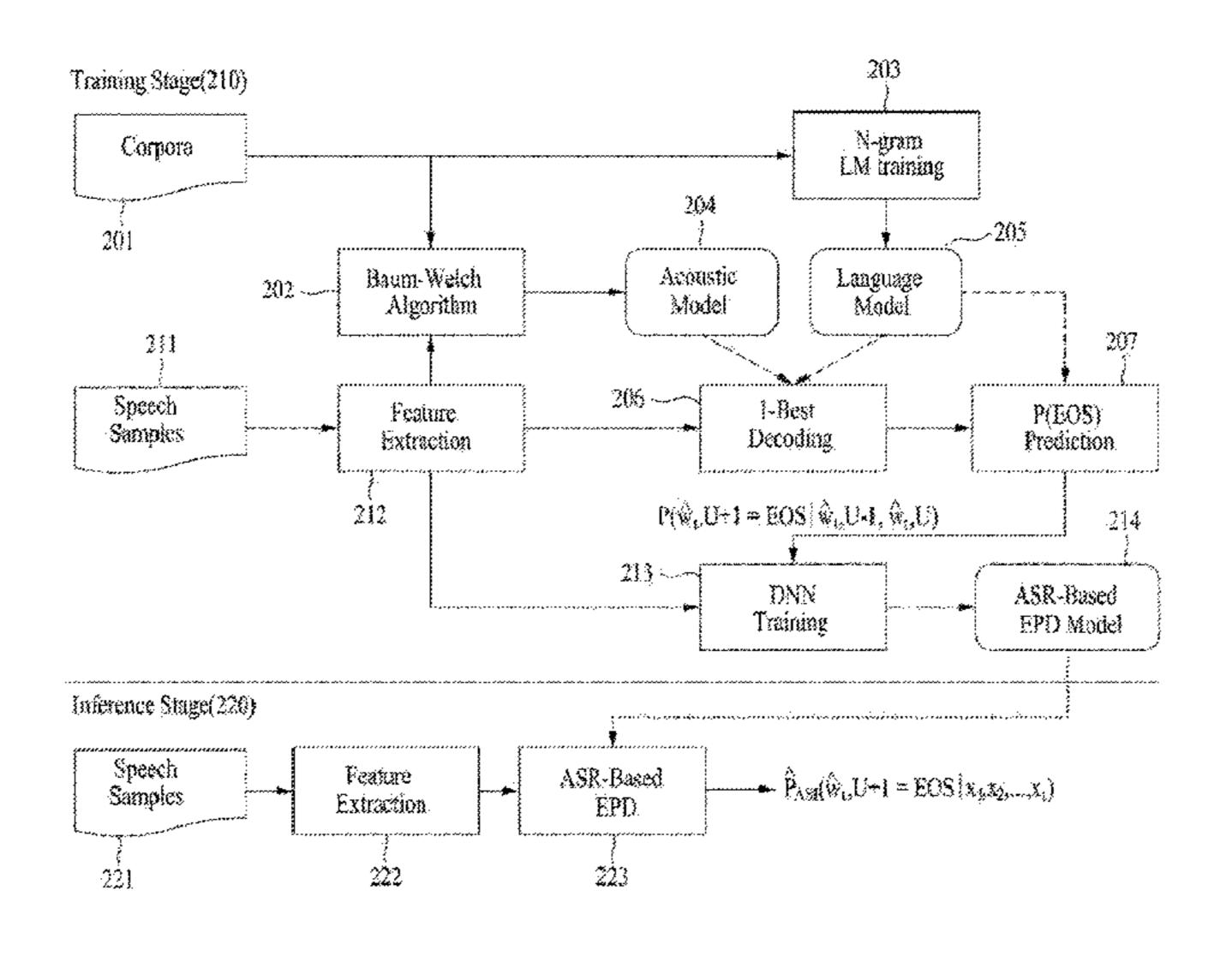
vector sequence extracted from a microphone input signal into an acoustic embedding extraction unit, and a decoder embedding extraction unit, which are based on a recurrent neural network (RNN); combining acoustic embedding, phonemic embedding, and decoder embedding to configure a feature vector by the acoustic embedding extraction unit, the phonemic embedding extraction unit; and inputting the combined feature vector into a deep neural network (DNN)-based classifier to detect a voice end point.
