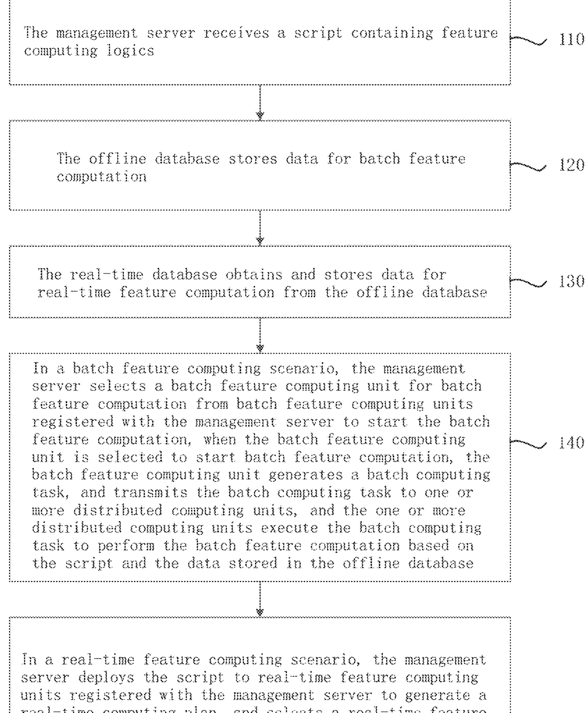
real-time computing plan, and selects a real-time feature computing unit used when executing the real-time computing plan from the real-time feature computing units registered with the management server, and when the real-time feature computing unit is selected to execute the real-time computing plan, the selected real-time feature computing unit performs the real-time feature computation based on the data stored in the real-time database and the script
