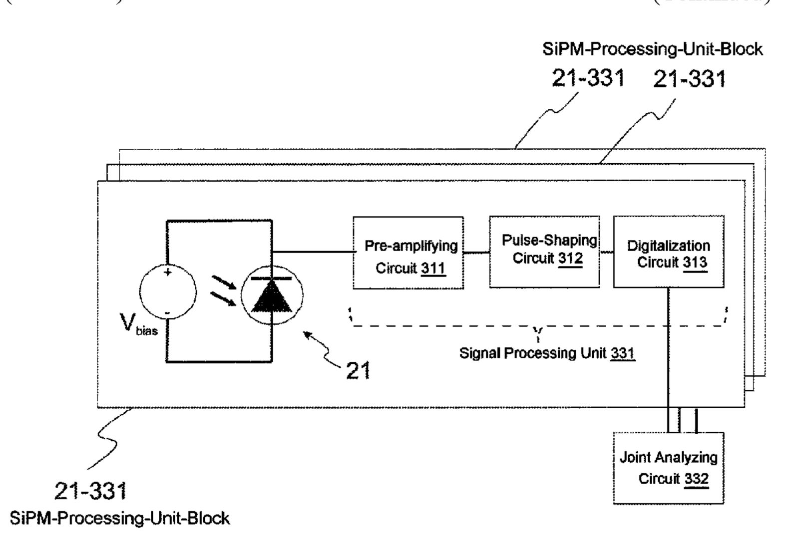
multiplier sensors, wherein the signal processing units each comprise a digitization circuit configured to generate a digitized signal for signal analysis by executing 1-bit digitization of a detection signal generated by at least one of the silicon photomultiplier sensors responsive to the detected scintillation light for determining the energy of the detected radiation event(s).
