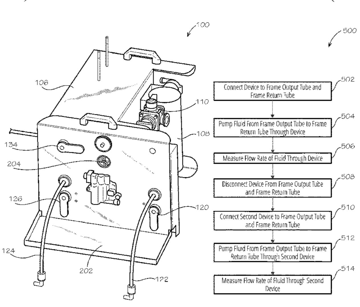
and the frame return tube, pumping a fluid from the frame output tube to the frame return tube through the device, and measuring a flow rate of the fluid through the device.
