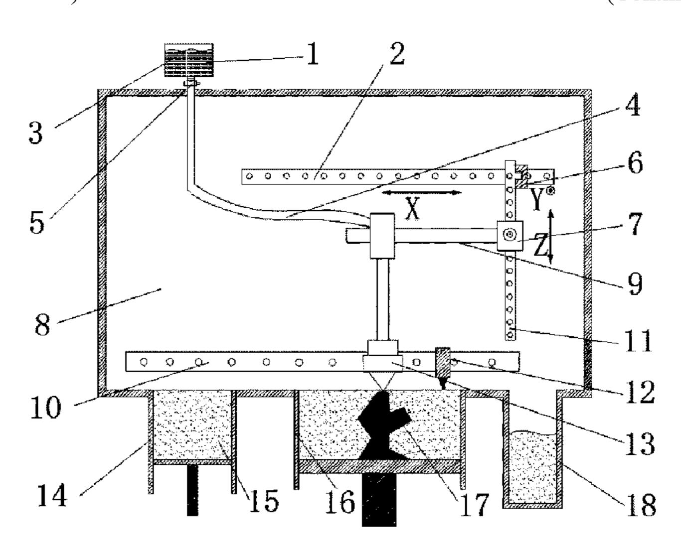
layer-by-layer cumulative stacking with existing 3D printing additive manufacturing equipment, and after solidification, the entire part is finally formed.
