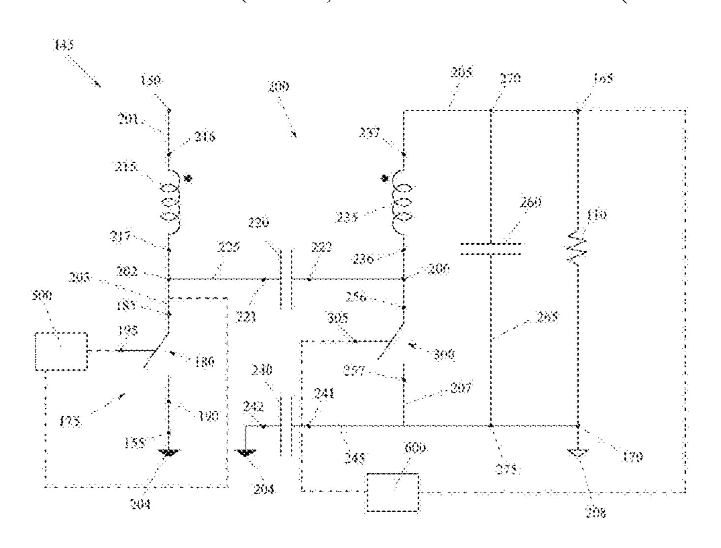
(201), a second resonance inductor (235) placed on the third electric branch (205), and a first resonance capacitance (220, 285, 290), wherein the first resonance inductor (215) and the second resonance inductor (235) are inductively coupled together with a reciprocal coupling factor less than 1.
