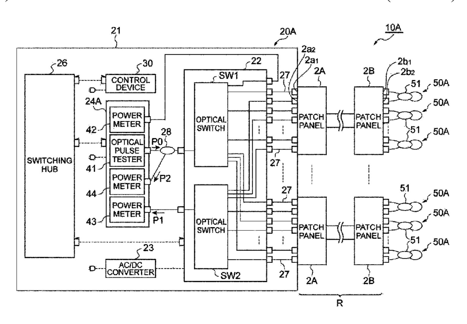
second optical fiber line of the pair of optical fiber lines includes a third end and a fourth end, the one or plurality of connection members optically connect the second end to the fourth end, the light source causes testing light to be incident on the first end, and the first power meter measures first intensity of first output light output from the third end by causing the testing light to propagate through the pair of optical fiber lines.
