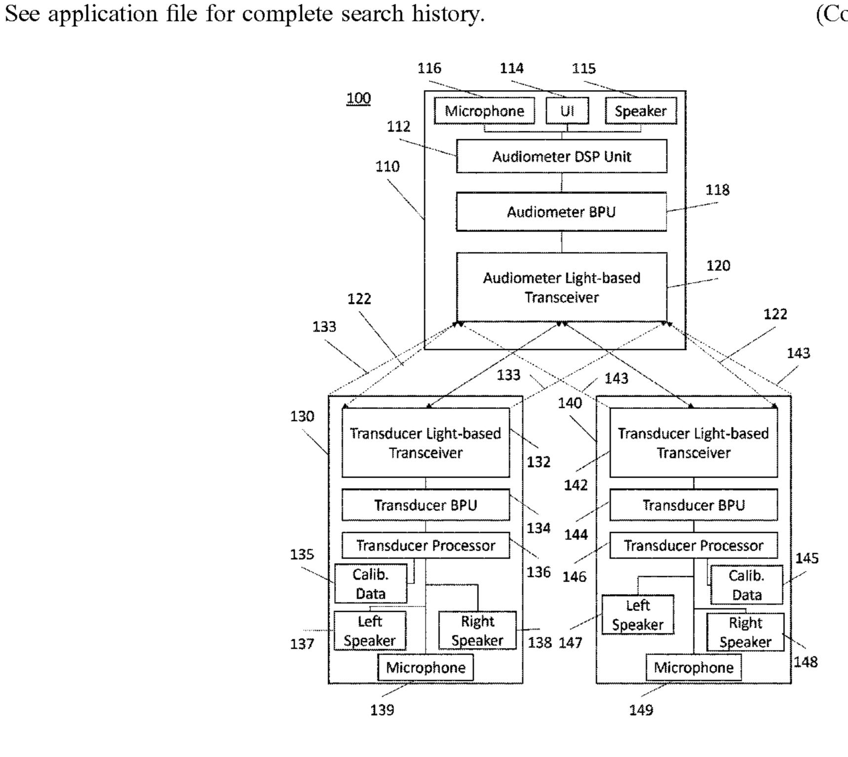
audiometer light-based transceiver. The system further includes a transducer including a transducer light-based transceiver in optical communication with the audiometer light-based transceiver, a transducer baseband processing unit, a transducer processor unit, and an audio speaker.
