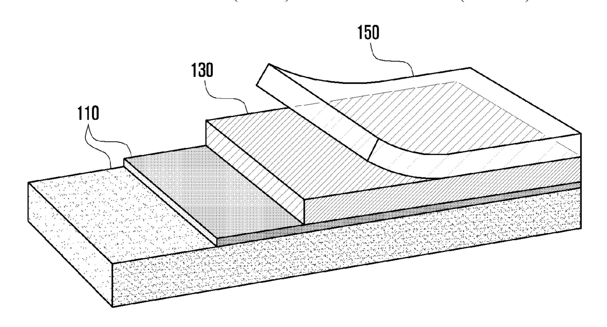
the first shield member, which is exposed between the first insulation layer and the second shield layer of the first shield member is covered.
