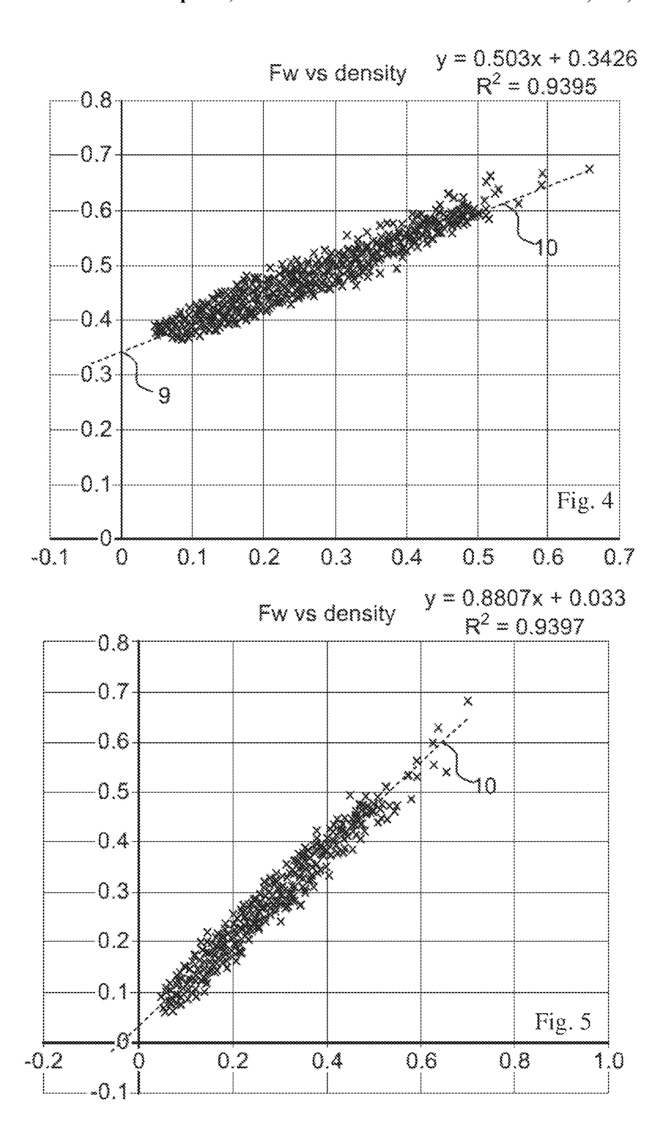
SYSTEM AND METHOD FOR MEASURING A MULTIPHASE FLOW BY MEASURING DENSITY AND ELECTRICAL IMPEDANCE FOR CORRECTING THE MEASUREMENT DUE TO EFFECT OF DEPOSITS ON INNER SURFACE OF PIPE WALLS
