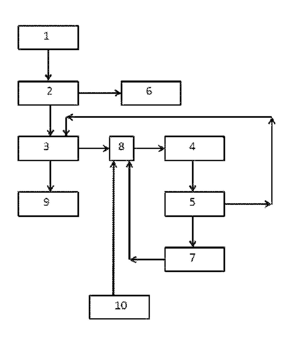
distribution of a quenching liquid is located and connected between the granulation section and the scrubbing section and the quenching section is connected to a quenching liquid providing section and the second condensation section.
