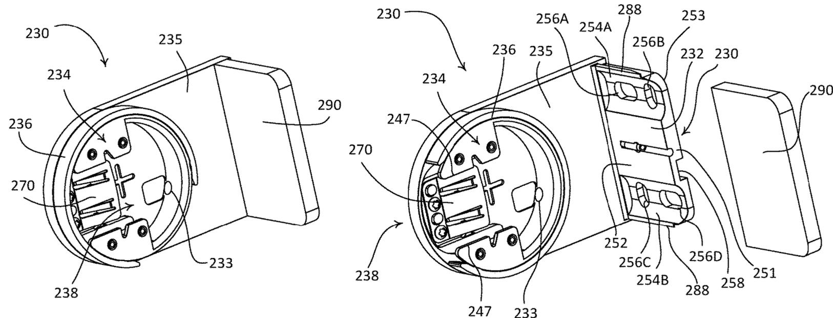
sliding cover that is configured to cover an access opening of the channel.
