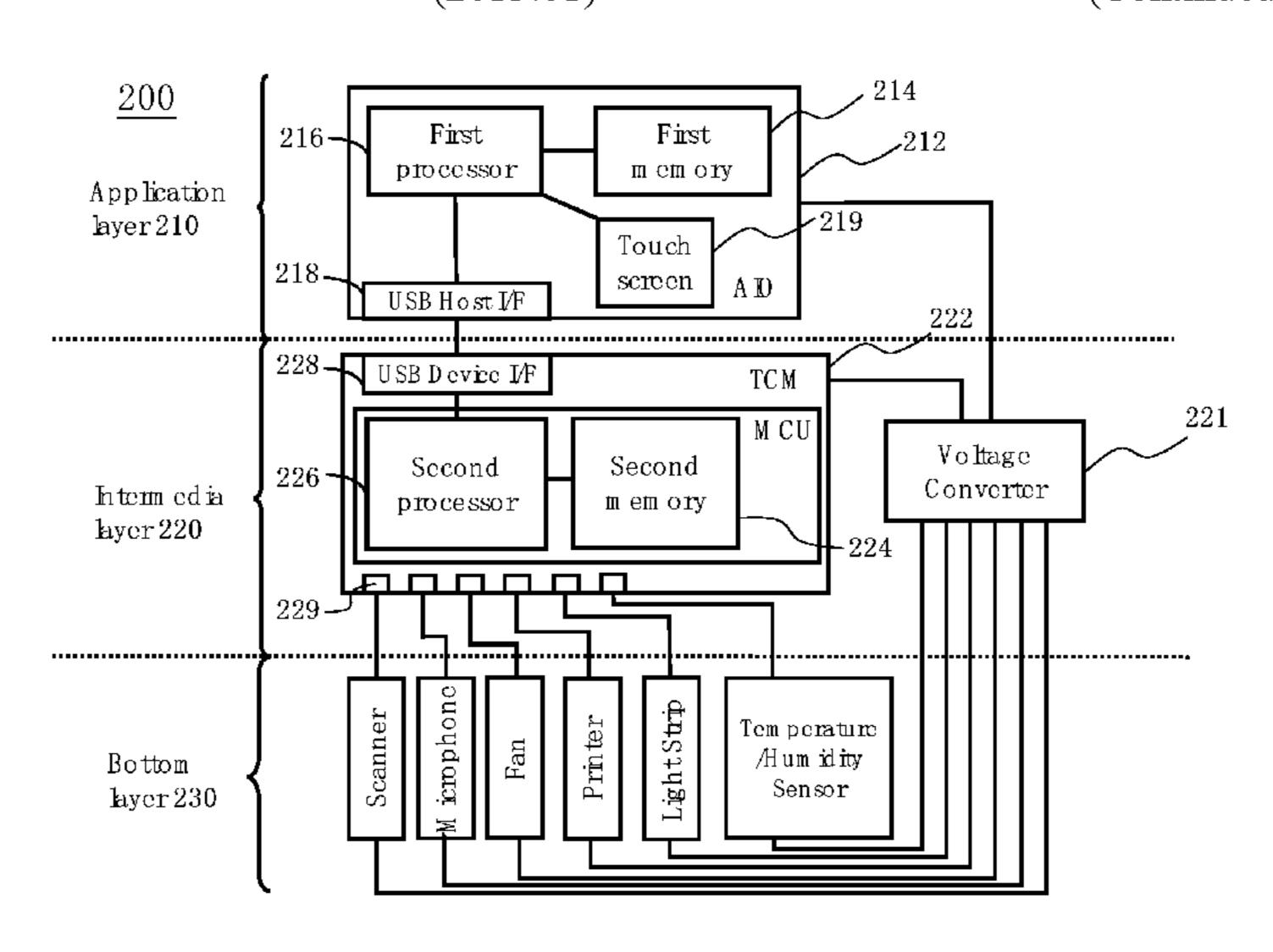
executes a control program stored in the second memory to control operations of the peripheral devices based on an instruction from the application-layer device. The peripheral devices do not communicate with the application-layer device directly.
