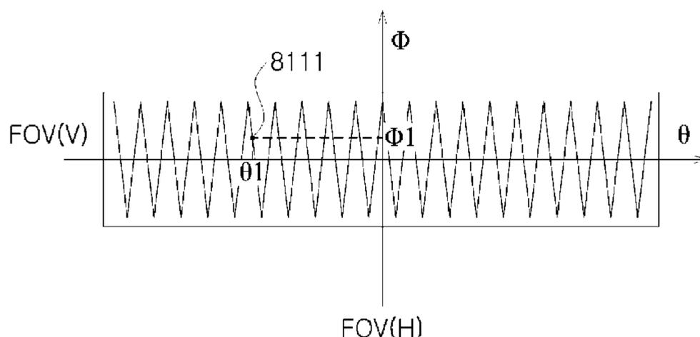
range, and wherein the second scanner comprises a rotating polygon mirror which changes the travel path of the laser which has the line-shaped irradiation area by rotating on one axis so as to extend the irradiation area to a plane shape.
