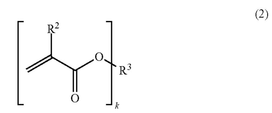
wherein k is an integer of 2 to 4, R<sup>3</sup> is a k-valent hydrocarbon group optionally having a heteroatom, and R<sup>2</sup> is a hydrogen atom or a methyl group.
