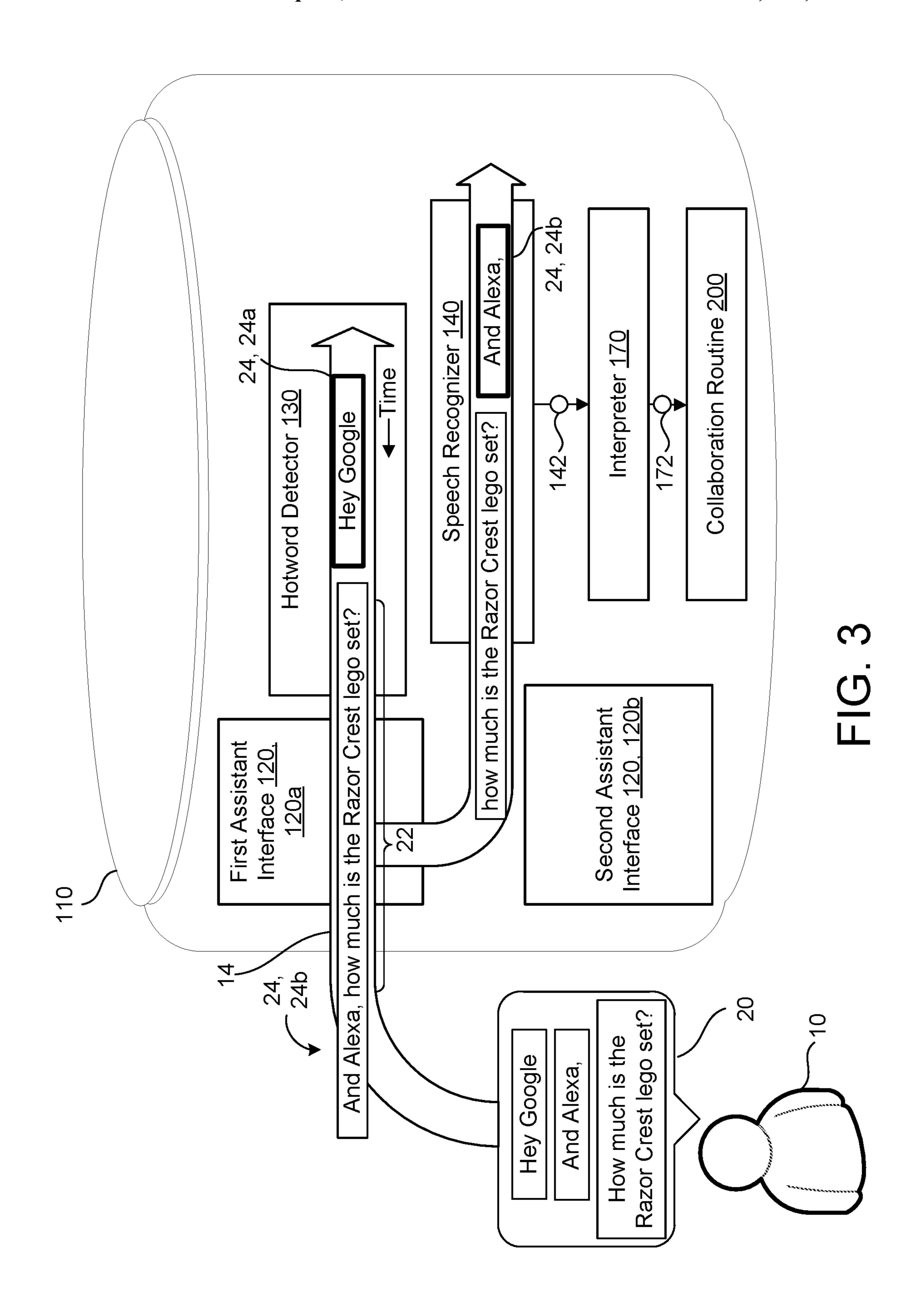
Receiving, At A First Assistant-enabled Device (AED), Audio Data Corresponding To An Utterance Spoken By The User And Directed Toward The First AED And A Second AED Among Two Or More AEDs Associated With The User, The Audio Data Comprising A Query Specifying An Operation To Perform
