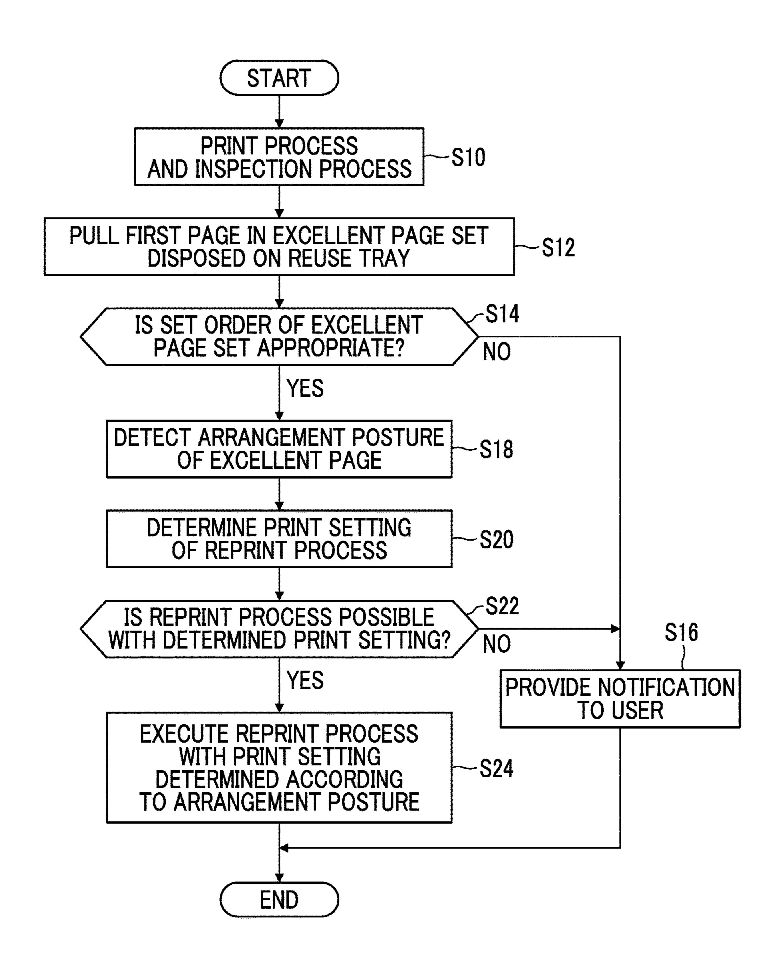
IMAGE FORMING APPARATUS AND NON-TRANSITORY COMPUTER READABLE MEDIUM STORING IMAGE FORMING PROGRAM CAPABLE OF PERFORMING REPRINT PROCESS FOR DEFECTIVE PAGES AND OUTPUTTING REPRINT PAGES TOGETHER WITH PAGES OF GOOD PRINT RESULTS
