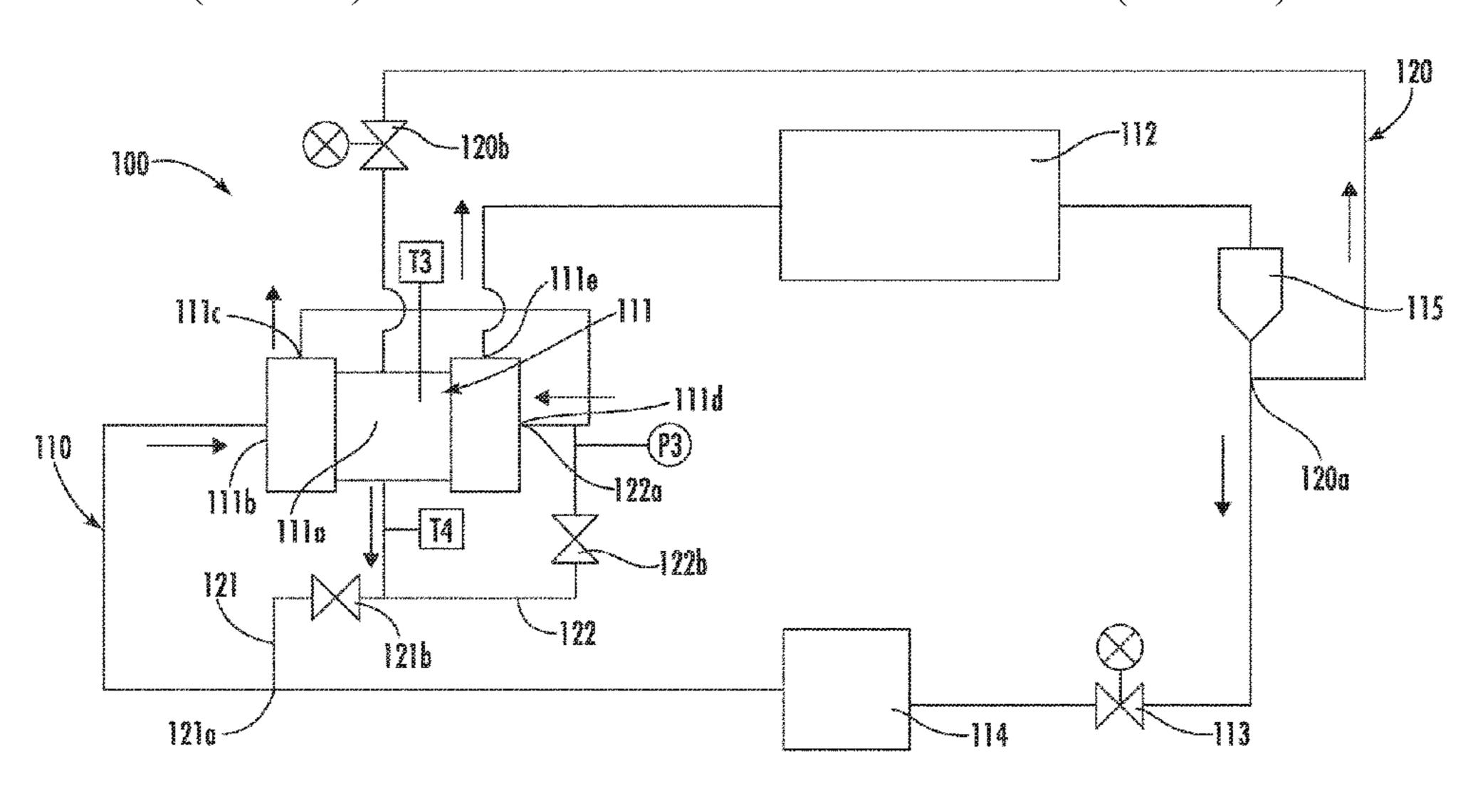
regulating valve on the cooling branch based on the temperature of the outlet downstream of the drive motor on the cooling branch and the intermediate suction pressure of the intermediate-stage suction port of the multi-stage compressor.
