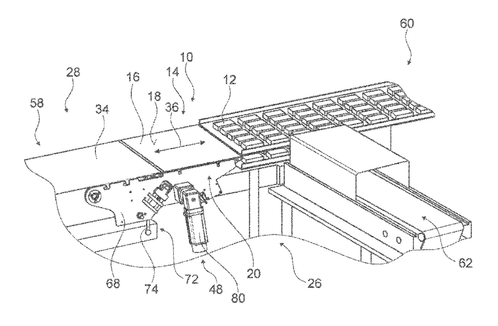
element (32) for guiding, in particular deflecting, an endless further transport element (34), in particular an endless further conveyor belt, wherein for the purpose of guiding the transport element (16) the further guide element (32) is supported by means of the bearing unit (24) so that it can be pivoted or tilted together with the guide element (22) and with the transport unit (14) relative to the frame unit (26).
